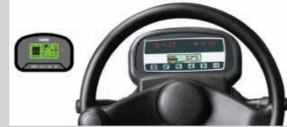
New Multi-Display employed full dotted LCD is located on the steering column to improve visibility and manipulate-ability.
