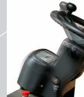
The adjustable steering Column ensure a comfortable working position.
